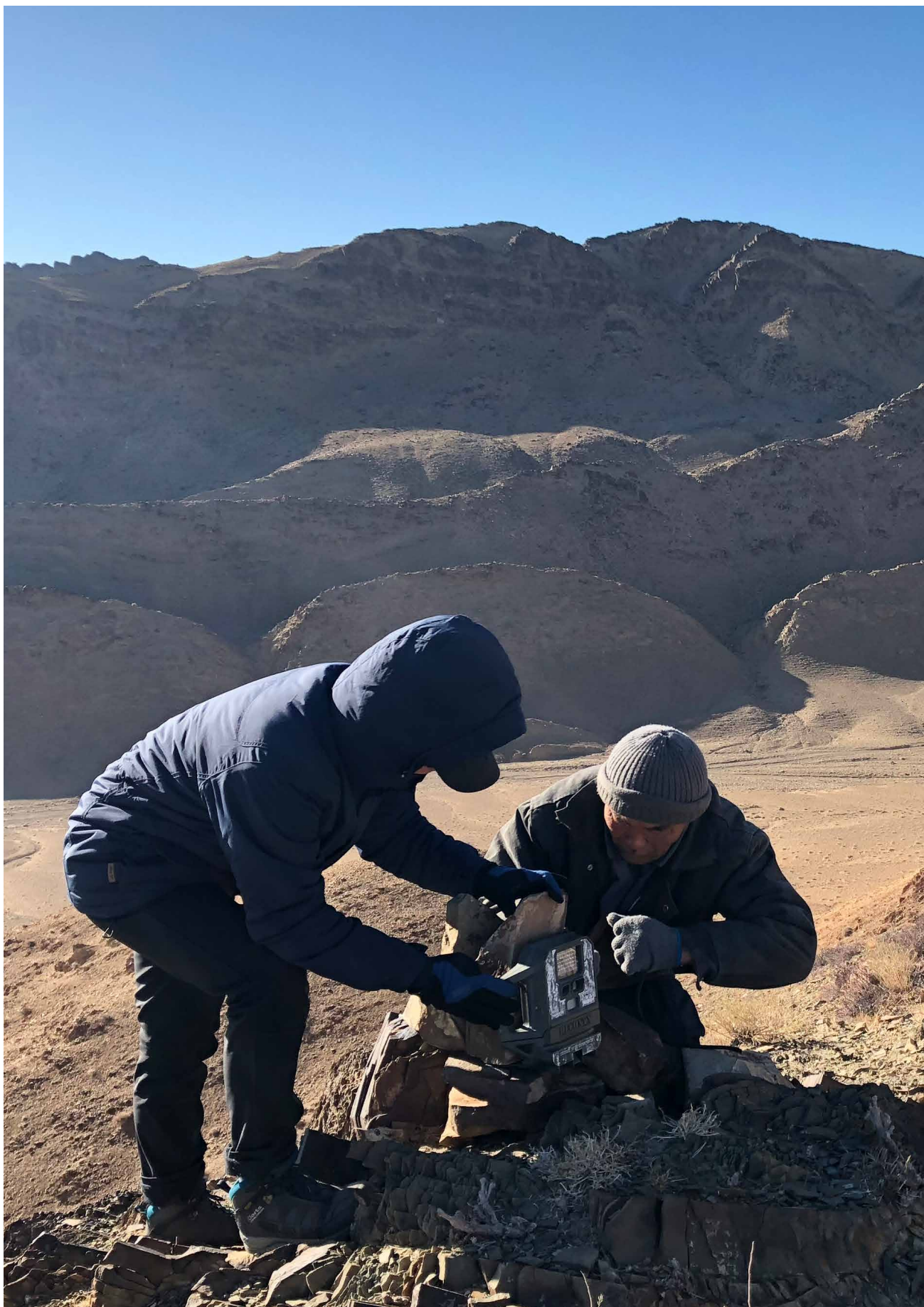
Camera traps are typically installed at locations that have high chance of snow movement of snow leopards such as saddles on ridgelines, cliff bases, overhanging rocks and canyons.
